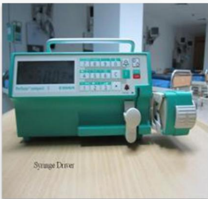
Syringe Driver Use to gradually administer small amount of fluids (with or without medication) to a patient
