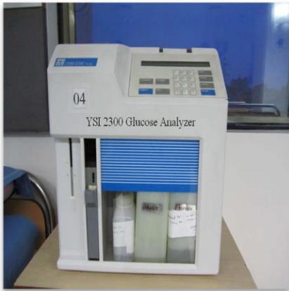
YSI 2300 Glucose Analyser Blood glucose measurement
